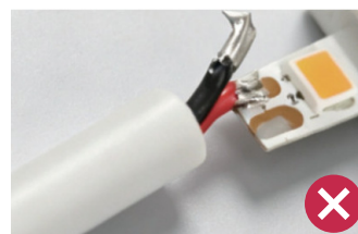
Incorrect: poor joint. Inspect joint strength.
