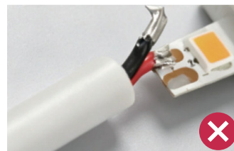
Incorrect: poor joint. Inspect joint strength.
