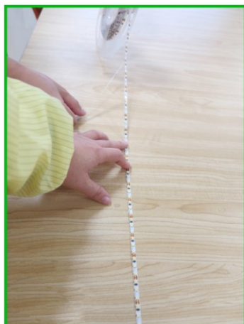
Support while unreeling
