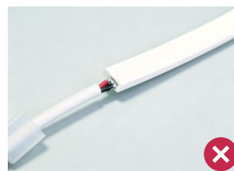
Incorrect: solder burr. Avoid shorts and bridges.
