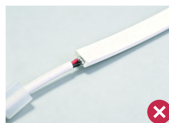
Incorrect: solder burr. Avoid shorts and bridges.
