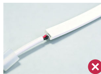
Incorrect: solder burr. Avoid shorts and bridges.
