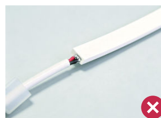
Incorrect: solder burr. Avoid shorts and bridges.
