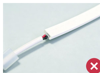
Incorrect: solder burr
